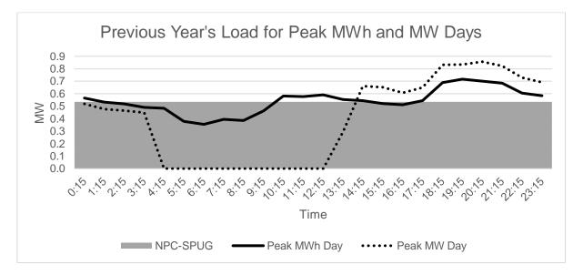
Peak MW occurred on 20:15 of June 18, 2019 due to heavy usage of electricity on summer/ dry season. Peak daily MWh occurred on 19:15 of May 5, 2019 due to usage of electricity on night time during summer season. As shown in the Load Curves, the available supply is lower than the Peak Demand.
