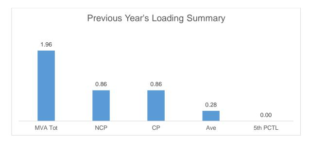
The Non-coincident Peak Demand is 0.86 MW, which is around 45.23% of the total substation capacity of 1.96 MVA at a power factor of 0.97. The load factor or the ratio between the Average Load of 0.28 MW and the Non-coincident Peak Demand is 33% of. A safe estimate of the true minimum load is the fifth percentile load of 0 MW which is 0% of the Non-coincident Peak Demand.
