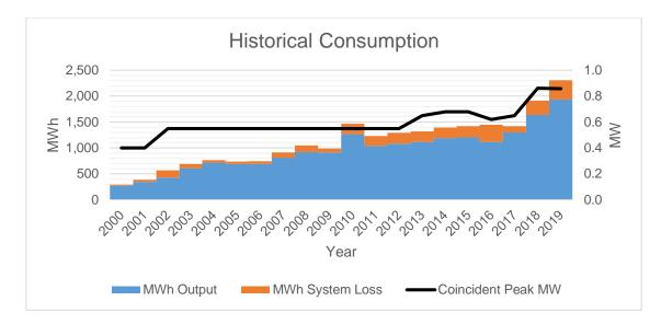
MWh Output increased from year 2017 to year 2018 at a rate of 25.85%, while MWh System Loss increased at a rate of 74.19% within the same period.
