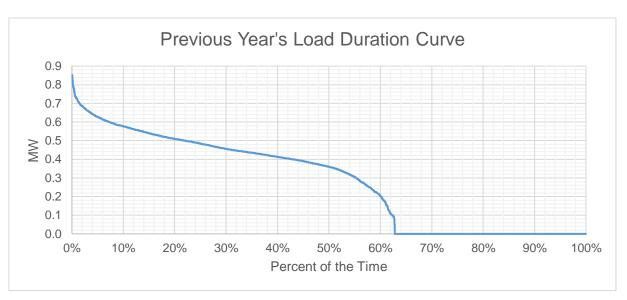
Based on the Load Duration Curve, the minimum load is 0.30 MW and the maximum load is 0.857 MW for the last historical year.
